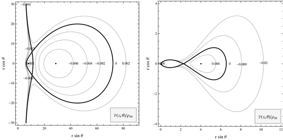
**Figure 1.** Charged Newtonian tori with cusps. The left panel shows negatively charged torus with cusps out of the equator (physically relevant torus is the small one on the *left*), while the *right* panel shows positively charged torus with the cusp in the equator.
